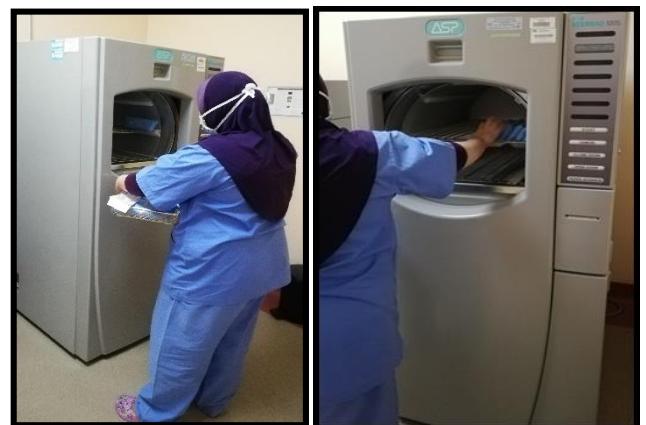
Gambar 9 & 10: Kaedah pensterilan set / peralatan menggunakan Vaporised Hydrogen Peroxide (Plasma) – Low Temperature
