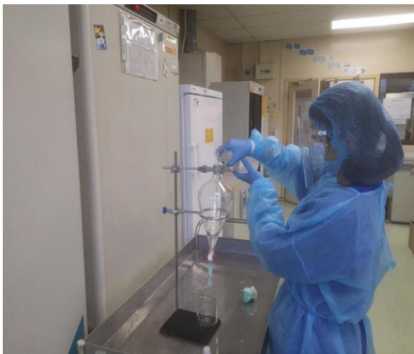
Pouring sample into a separating funnel using chiller for overnight incubation at 4°C)
