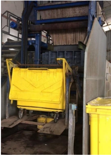
Vials uploaded into the Amb EcoSteryl Microwave Disinfectant System
